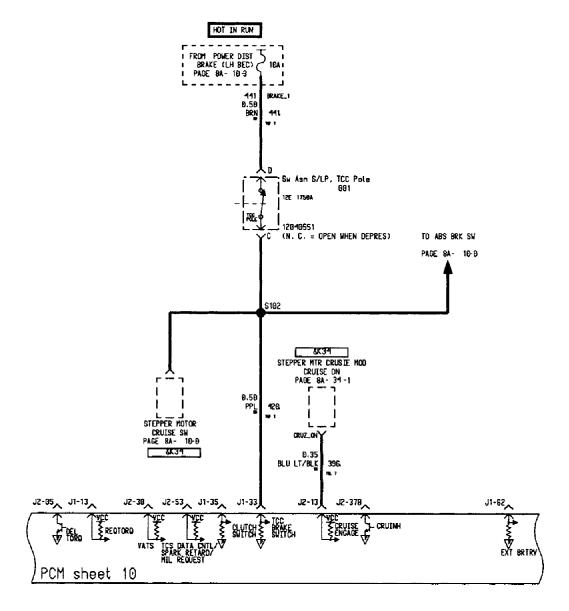
Figure 3.2.1a - VI - P/Truck - Mechanization Diagram - TCC Switch & Cruise Control
